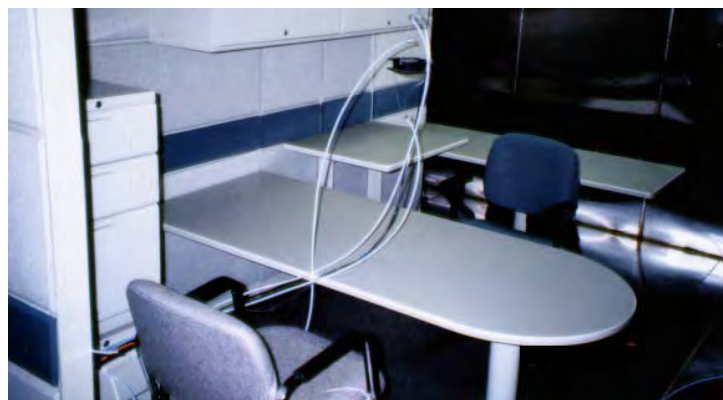
Figure 5.1-O Office Workstation Test: 1942 ft 3 (55 m 3 ) Emissions Chamber Photograph copyright NRC.
