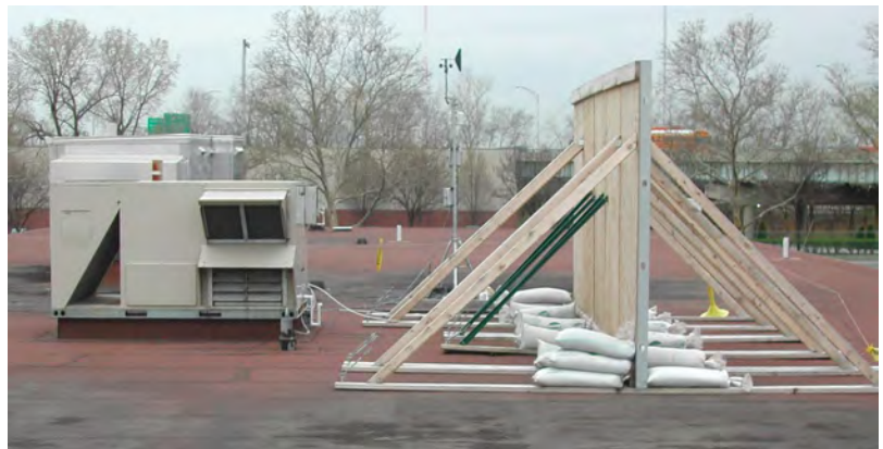
Figure 3.2-I Side Wall Obstruction for Packaged HVAC Test Unit—Wall Installed 10 ft (3 m) from Unit Photograph copyright Battelle Memorial Institute.
