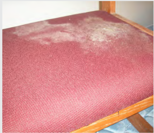
Figure 2.3-B Mold Growth due to Negative Pressure
