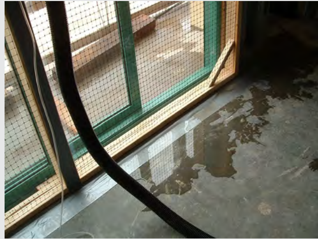
Figure 1.2-J Water Leakage Failure—Early Test Unit Photograph courtesy of Dave MacPhaul; copyright CH2M HILL.
