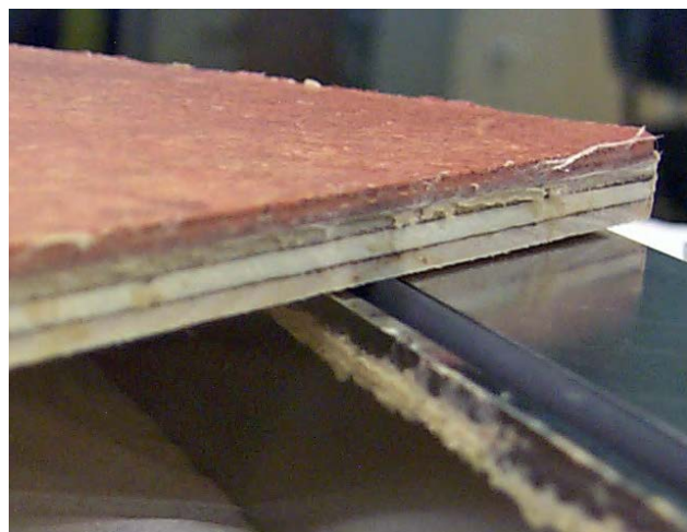
Figure 5.1-H Linoleum/Adhesive/ Plywood Tested as an Assembly Photograph copyright NRC.
