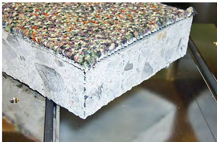
Figure 5.1-I Carpet/Adhesive/Concrete Test Assembly Photograph copyright NRC.
