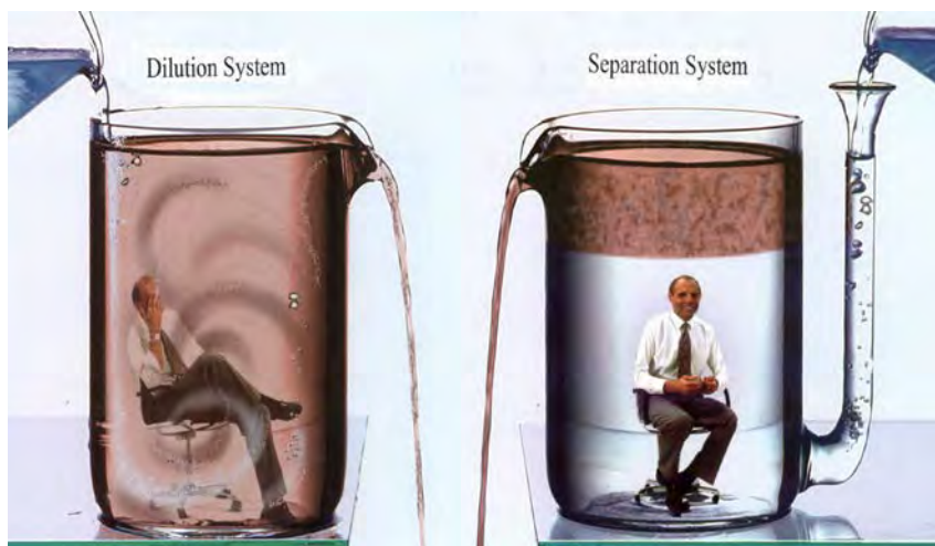
Figure 1.3-E Visual Representation of Displacement Ventilation Graphic copyright Healthy Buildings International, Inc., used with permission.
