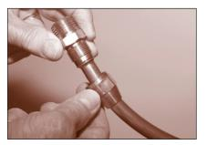
FIGURE 28: Flare Fitting/Flared Joint During Assembly
