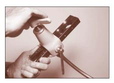
FIGURE 31: Lowering the Flaring Cone into the Tube End
