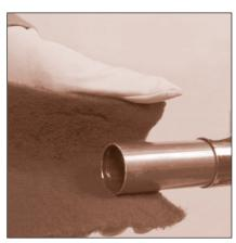
FIGURE 16: Cleaning: Abrasive Pad
