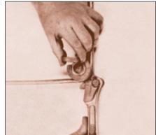
FIGURE 9: Bending Using a Lever-Type Hand Bender (tool shown
