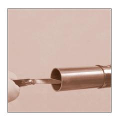
FIGURE 13: Reaming: Pocket Knife
