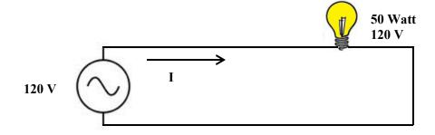
8. Determine the resistance of the 150-Watt lamp and the total current in the circuit shown below.
