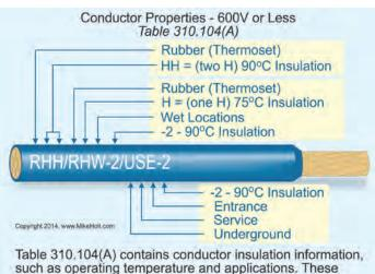
conductors can be used in any Chapter 3 wiring method.
