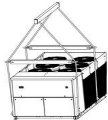
Figure 168: lifting the chiller unit
