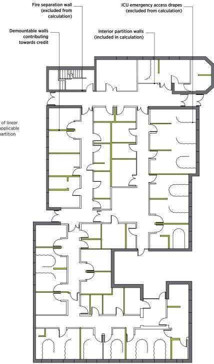
Figure 5. Example of linear surface locations applicable for demountable partition calculation
