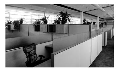
**Figure 8.** Partial-height partitions with frosted glass. Frosted glass is not acceptable because it interferes with occupants' views to the vision glazing. Photo by Marcus Sheffer.
